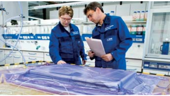
The Baxxodur application laboratory at the Ludwigshafen, Germany, site with large-scale heating tables, infusion and injection units to simulate a variety of processing conditions prevailing at customer facilities.
