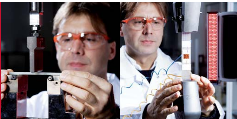
Three-point bend test according to DIN EN ISO 14125
